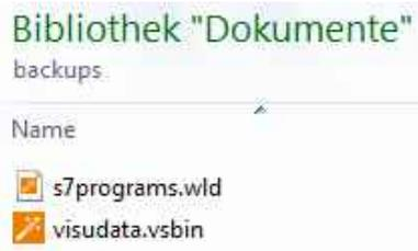
With these data S7-programs and visualizations can be updated by a Micro-SD-card only – complete without any PC. (more at „System functions“, chapter „Data backup and restore“)
